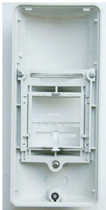
Fig. 12: PET Immunity Filter assembled
